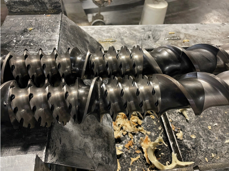
Above: A clean pair of compounding screws after removal of the Asaclean purge
