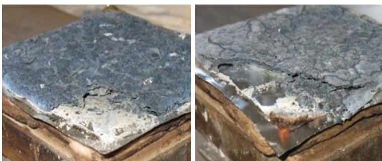
Above: Images showing the improved char formation resulting from the addition of 3% of Evonik’s Tegomer FR100 additive in a cable compound sample (right)
